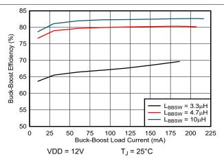
Figure 8-4. Buck-Boost Efficiency vs Load When I<sub>BBSW,PK</sub> = I<sub>BBSW,PK</sub>(high)
