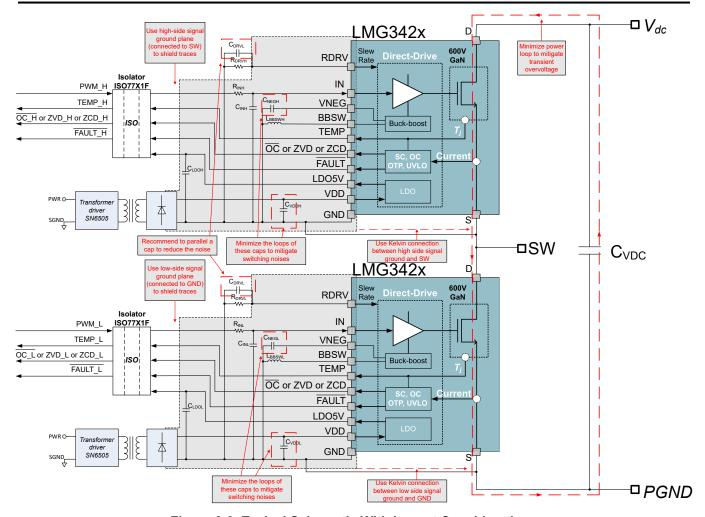
Figure 8-9. Typical Schematic With Layout Considerations
