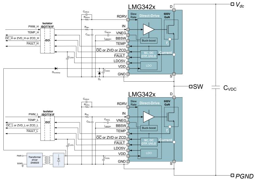
Figure 8-2. Typical Half-Bridge Application With Bootstrap
