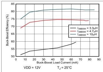
Figure 8-3. Buck-Boost Efficiency vs Load When  $I_{BBSW,PK} = I_{BBSW,PK(Iow)}$
