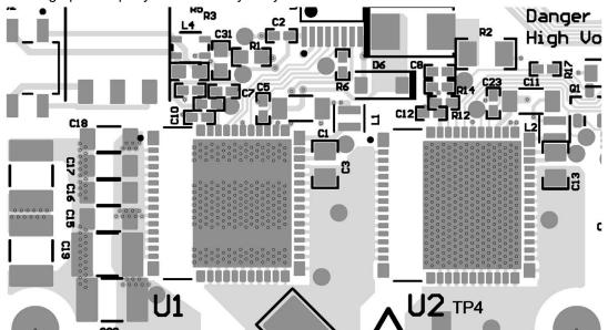
Figure 8-10. Half-Bridge Top-Layer Layout
