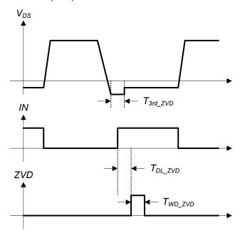
Figure 6-3. ZVD Timing Specifications
