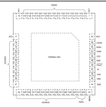
Figure 4-3. LMG3427R030 RQZ Package, 54-Pin VQFN (Top View)
