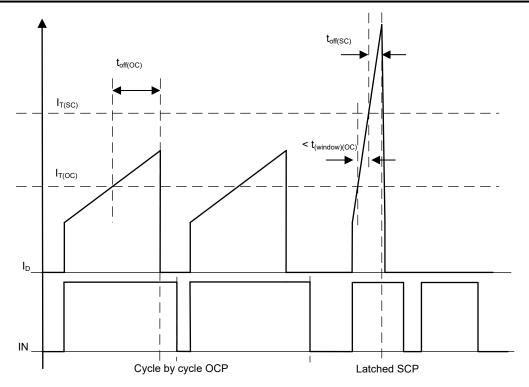
Figure 7-5. Overcurrent Detection vs Short-Circuit Detection
