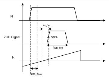
Figure 7-10. ZCD timing diagram when FET turns on into negative current
