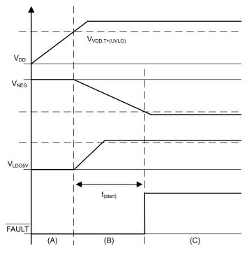
Figure 7-12. Start-Up Timing Diagram
