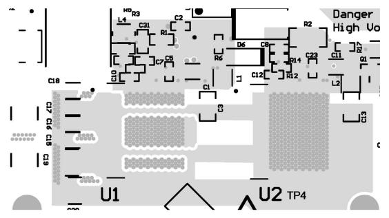
Figure 8-11. Half-Bridge Mid-Layer Layout
