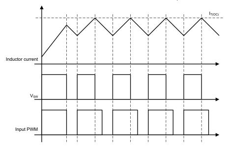
Figure 7-4. Cycle-by-Cycle OCP Operation
