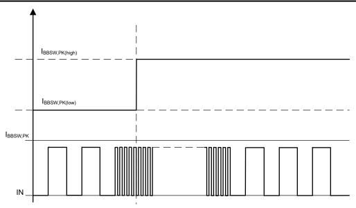
Figure 7-3. Buck-Boost Converter Peak Current
