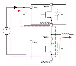
Figure 8-7. Charging Path for Bootstrap Diode
