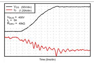
Figure 8-6. Turn-Off Waveform in Application Example
