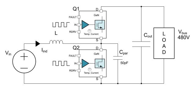
Figure 6-5. Circuit Used for SOA Curve
