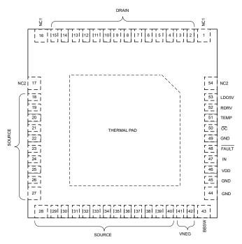
Figure 4-1. LMG3422R030 RQZ Package, 54-Pin VQFN (Top View)
