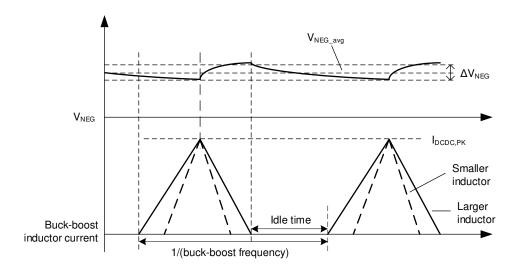
Figure 7-2. Buck-Boost Converter Inductor Current
