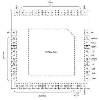
Figure 4-2. LMG3426R030 RQZ Package, 54-Pin VQFN (Top View)
