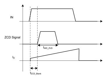
Figure 7-11. ZCD timing diagram when FET tuns on into positive current
