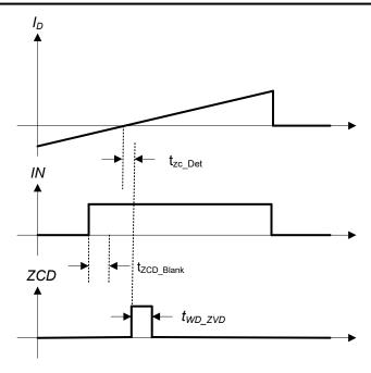
Figure 6-4. ZCD Timing Specifications
