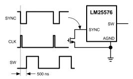
Figure 9. Sync from External Clock
