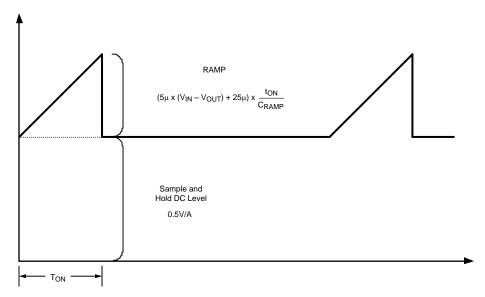
Figure 12. Composition of Current Sense Signal
