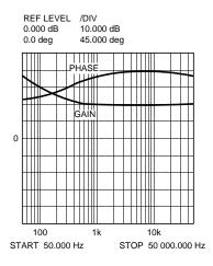
Figure 16. Error Amplifier Gain and Phase
