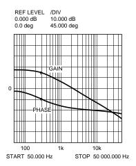
Figure 15. Gain and Phase of Modulator  $R_{LOAD} = 5$  Ohms and  $C_{OUT} = 177 \mu F$
