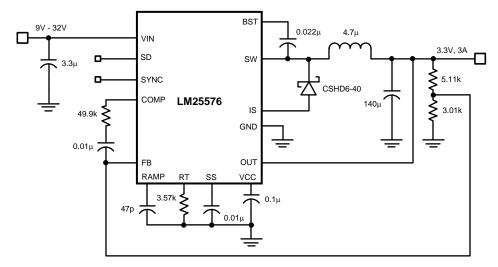
Figure 20. Schematic 3.3 V, 3 A, 1 MHz
