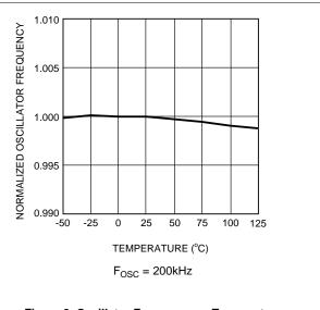
Figure 2. Oscillator Frequency vs Temperature
