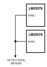
Figure 10. Sync from Multiple Devices
