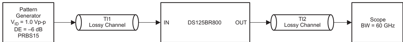
Figure 11. Test Setup Connections Diagram
