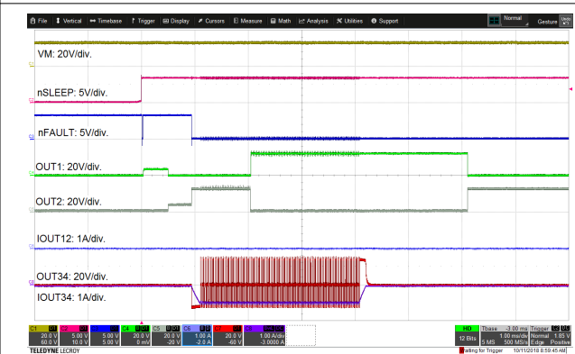
Figure 8-14. Open Load Detect Operation
