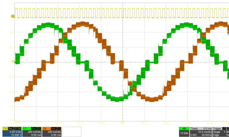
Figure 8-4. 1/8 Microstepping With smart tune Dynamic Decay
