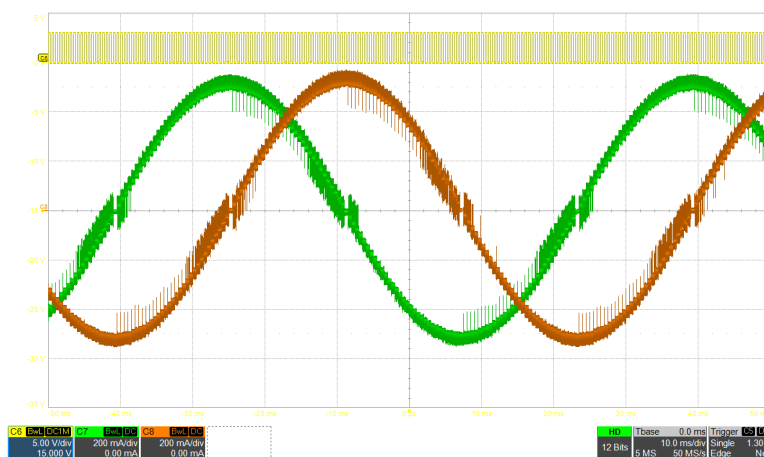
Figure 8-5. 1/32 Microstepping With smart tune Ripple Control Decay
