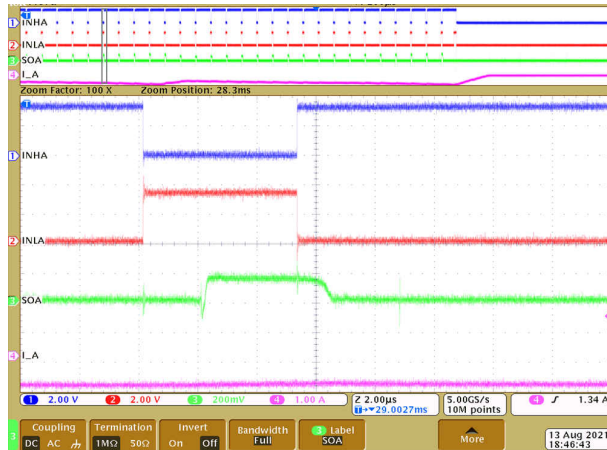
Figure 9-6. Driver PWM operation with feedback
