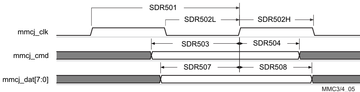
Figure 5-107. MMC/SD/SDIOj in - High-Speed SDR50 - Receiver Mode
