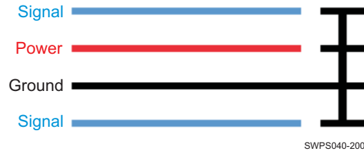
Figure 7-19. Guard Ring Routing
