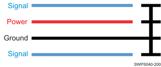
Figure 8-19. Guard Ring Routing
