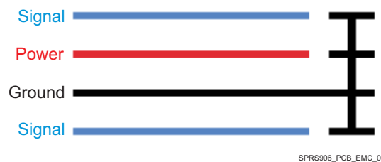
Figure 8-13. Guard Ring Routing
