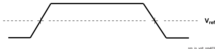
Figure 7-2. Input and Output Voltage Reference Levels for AC Timing Measurements
