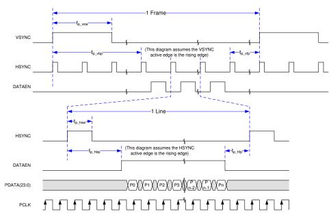
Figure 5-5. Source Frame Timing
