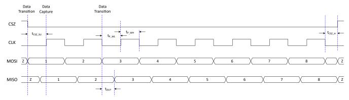
Figure 5-6. Host/Diagnostic Port SPI Interface Timing (Example: SPI Mode 0 (Clock Polarity = 0, Clock Phase = 0))
