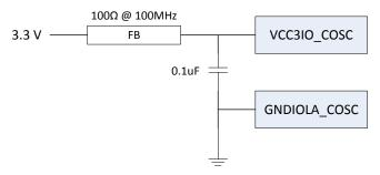
Figure 8-14. Crystal Power Supply Filtering
