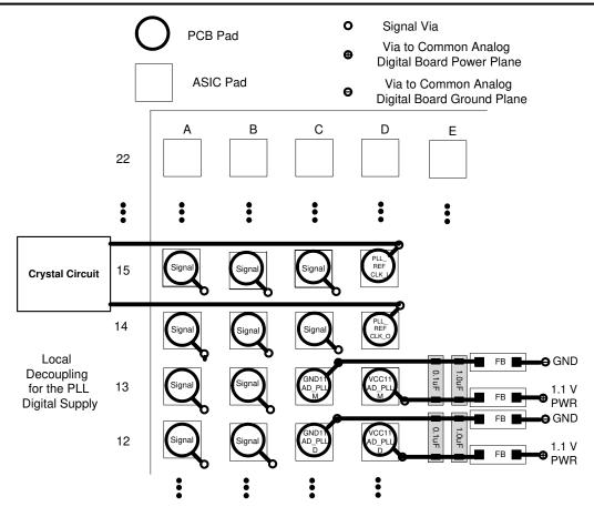
Figure 8-11. DLPC230-Q1 PLL Filter Layout
