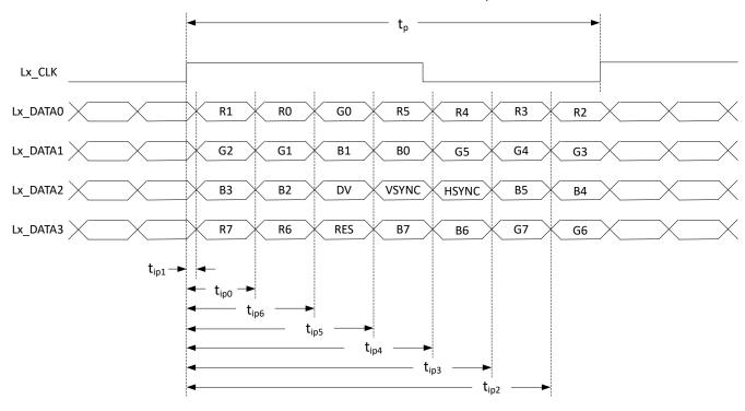
Figure 5-4. OpenLDI Interface Timing
