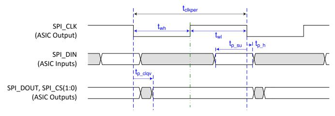
Figure 5-7. Flash Interface Timing
