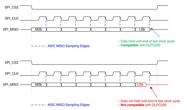
Figure 5-8. Flash Interface Data Capture Requirements
