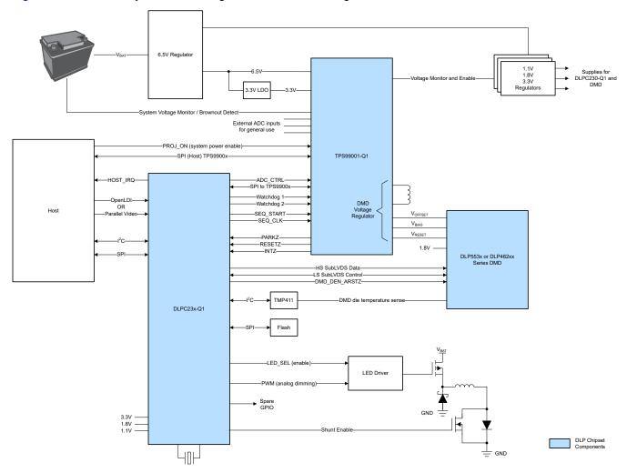
Figure 8-2. Headlight System Block Diagram
