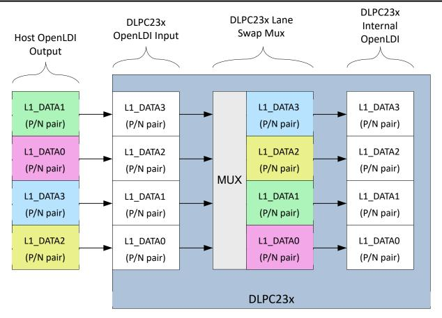
Figure 7-4. Example of Alternate OpenLDI Port Lane Mapping
