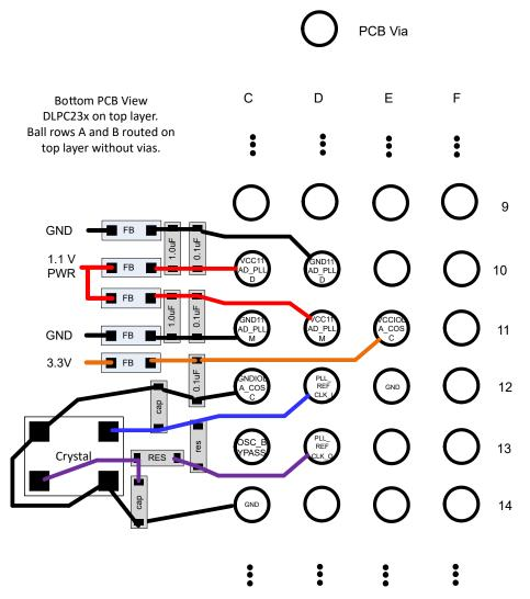
Figure 8-12. DLPC231-Q1 PLL Filter and Crystal Layout
