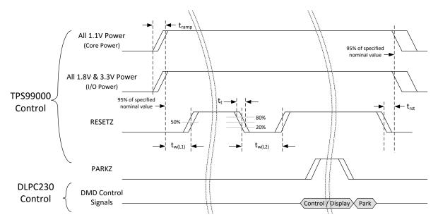
Figure 5-2. Power Supply and RESETZ Timing
