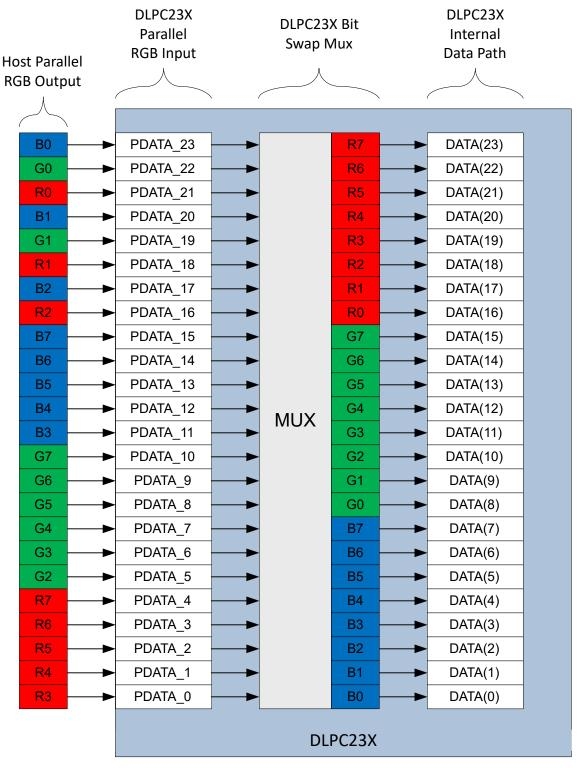
Figure 7-2. Example of Alternate Parallel Port Bit Mapping
