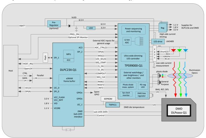
Figure 8-1. HUD System Block Diagram
