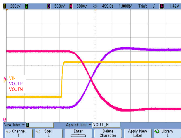
Figure 8-4. Step Response of the AMC1301-Q1
