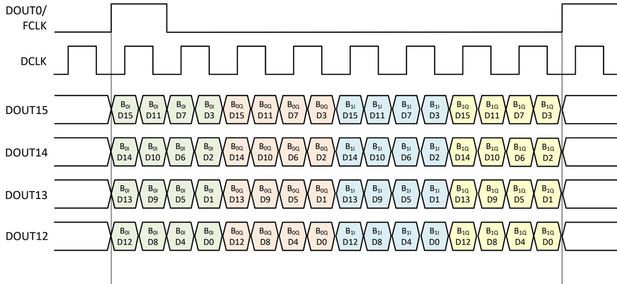
**Figure 8-60. SLVDS frame assembly for example 3**
