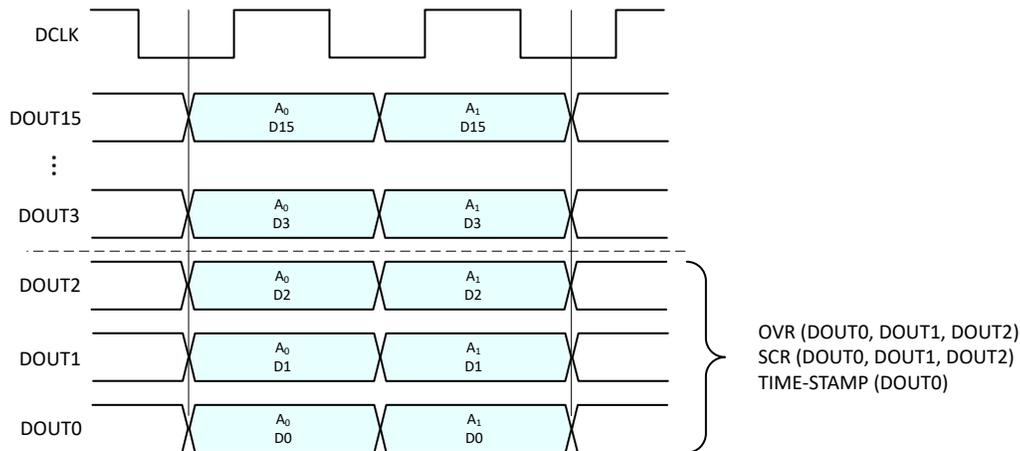
**Figure 8-56. Output data format in SDR LVDS mode**
