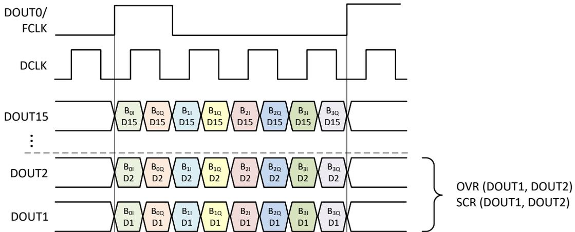
Figure 8-62. Output Data Substitution: 16 SLVDS Lanes
