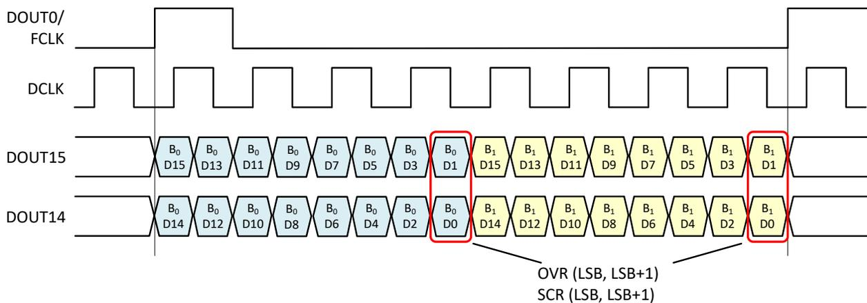
Figure 8-63. Output Data Substitution: <16 SLVDS Lanes
