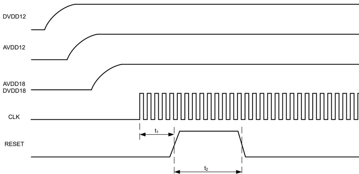
Figure 9-8. Initialization of Serial Registers After Power-Up
