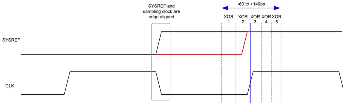
**Figure 8-18. Detection of SYSREF Transition Within Capture Window**
