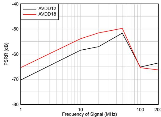
**Figure 9-9. Power Supply Rejection Ratio (PSRR) vs Frequency**
