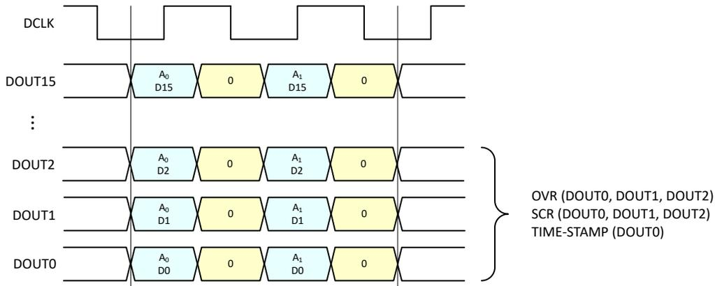
**Figure 8-57. Output data format in DDR LVDS mode**
