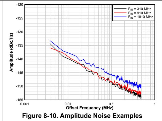
The internal clock noise is also dependent on the external clock amplitude. Figure 8-11 to Figure 8-14 show the expected AC performance at different input frequencies across clock amplitude.
