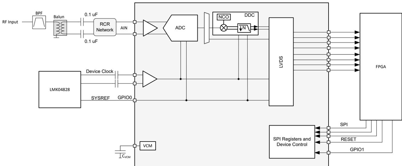
**Figure 9-1. Typical Configuration for Wideband Spectrum Analyzer**
