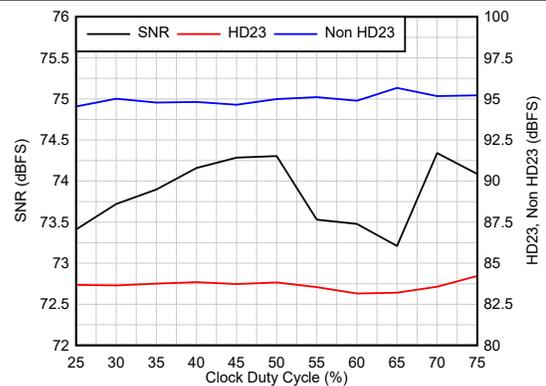
**Figure 6-18. AC Performance vs Clock Duty Cycle**
