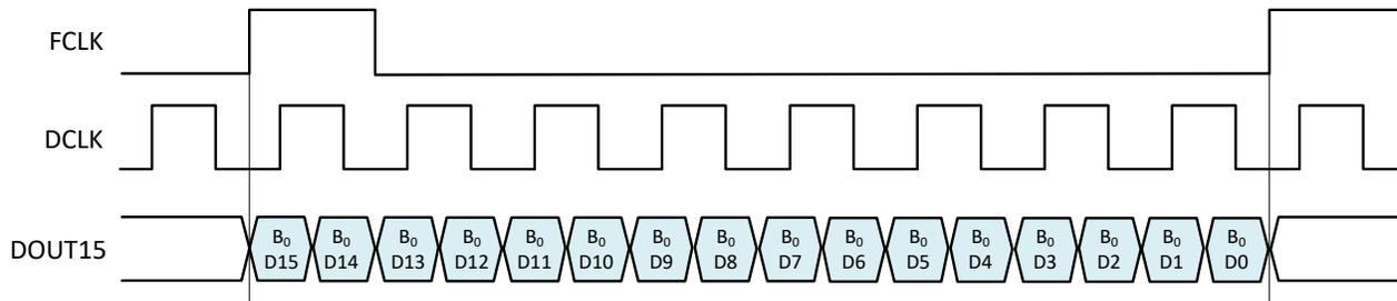
**Figure 8-58. SLVDS frame assembly for example 1**
