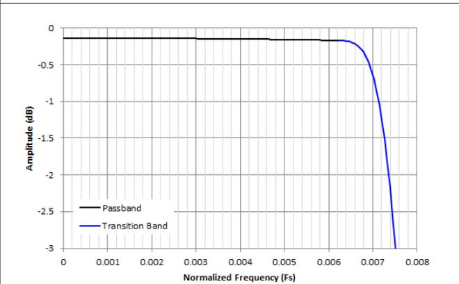
**Figure 8-35. Complex Decimation by 64 Filter Ripple Response**
