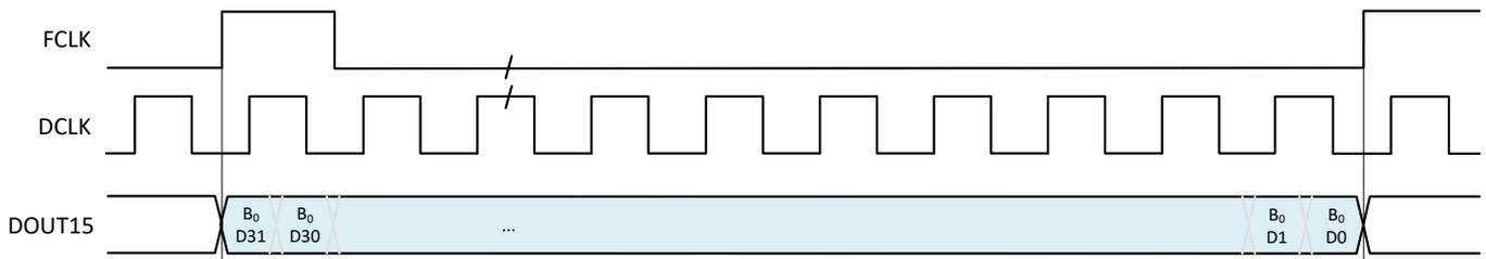
**Figure 8-59. SLVDS frame assembly for example 2**
