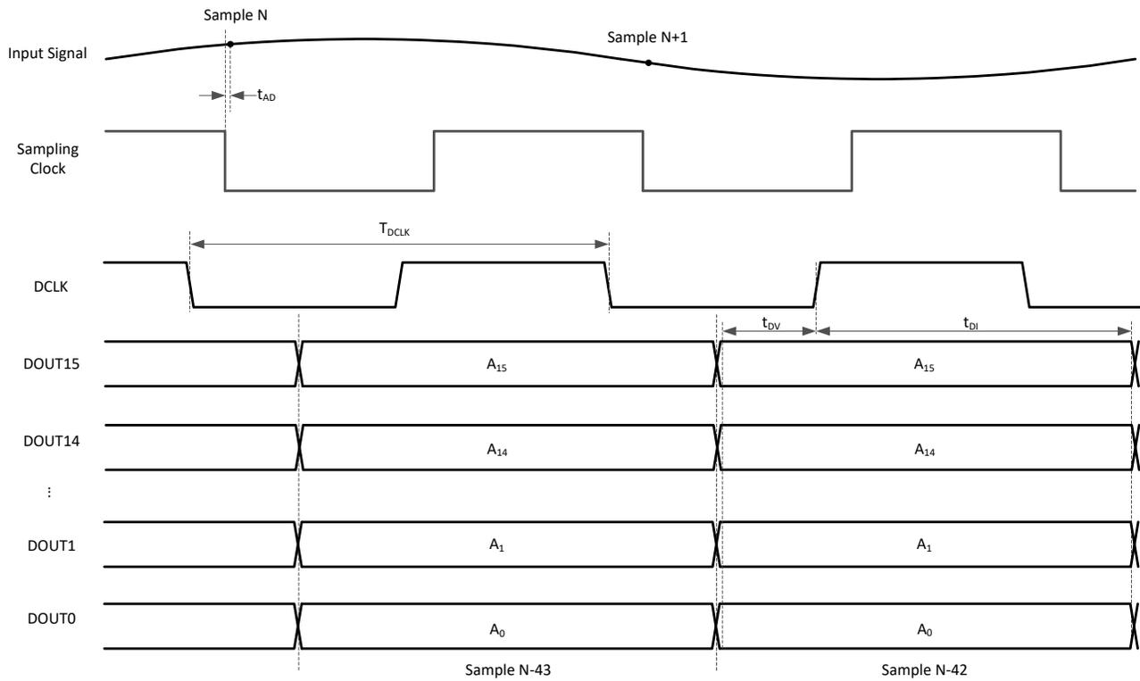
**Figure 7-1. Timing Diagram - Parallel SDR LVDS (default)**
