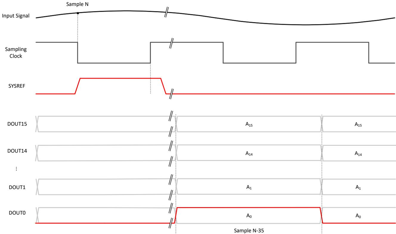
Figure 8-19. Timing Diagram - Time-Stamp Output with SDR LVDS
