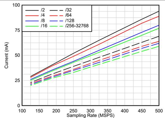
Figure 6-56. Current vs Sampling Rate
