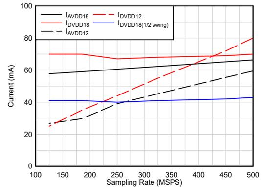
Figure 6-54. Current vs Sampling Rate
