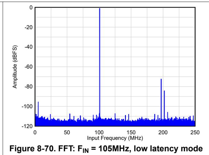
**Figure 8-70. FFT:  $F_{IN} = 105\text{MHz}$ , low latency mode**
