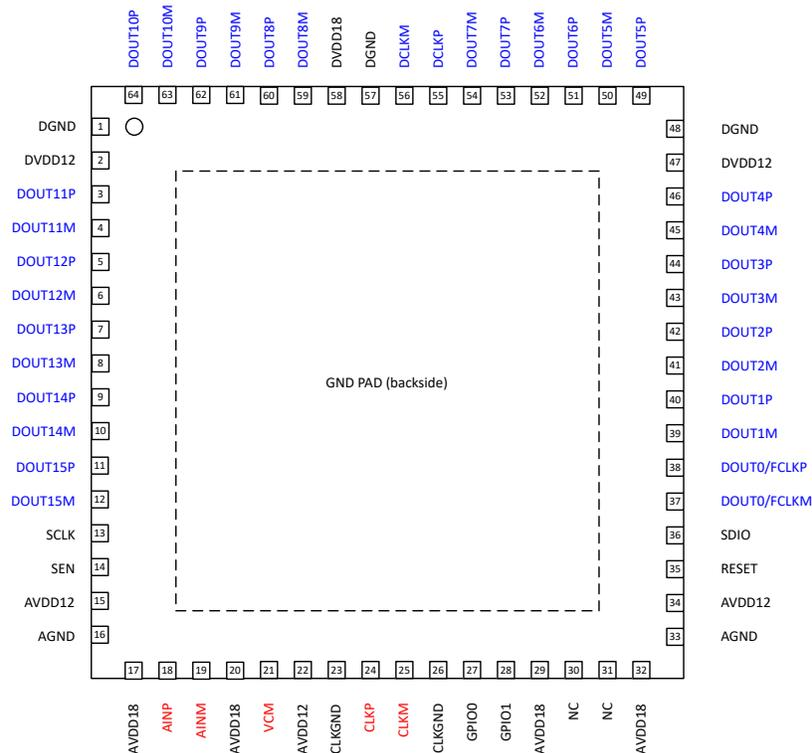
**Figure 5-1. RTD Package, 64 Pin VQFN (Top View)**
