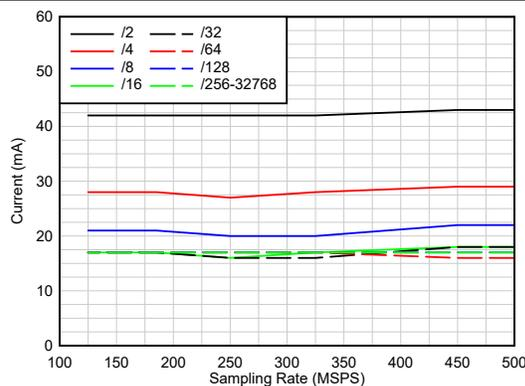
Figure 6-55. Current vs Sampling Rate
