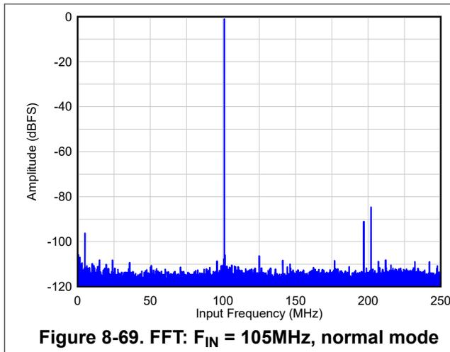
**Figure 8-69. FFT:  $F_{IN} = 105\text{MHz}$ , normal mode**
