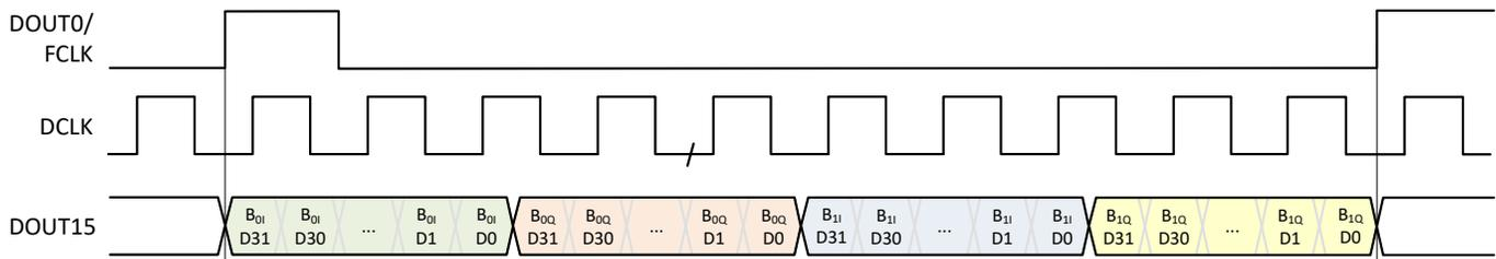
**Figure 8-61. SLVDS frame assembly for example 4**
