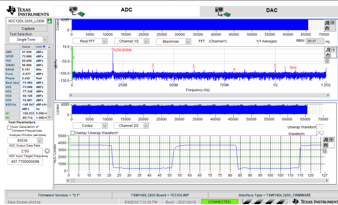
Figure 8-11. 200-MHz, Sine-Wave (Channel A) Frequency Domain (FFT) and 40-MHz, Square-Wave (Channel B) Time Domain for 5-GSPS, Single-Channel Oscilloscope
