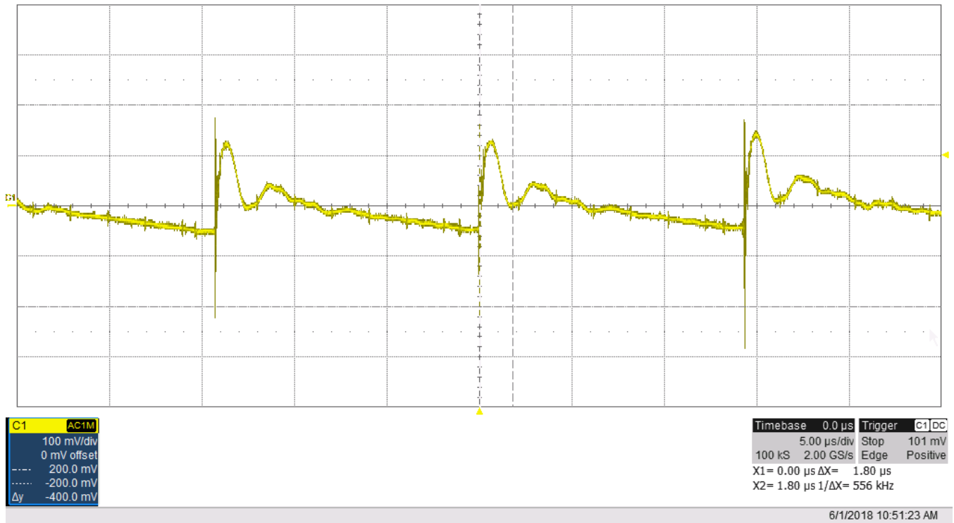
Figure 12. Output Ripple Voltage 12 V Output and 230 VAC Input
