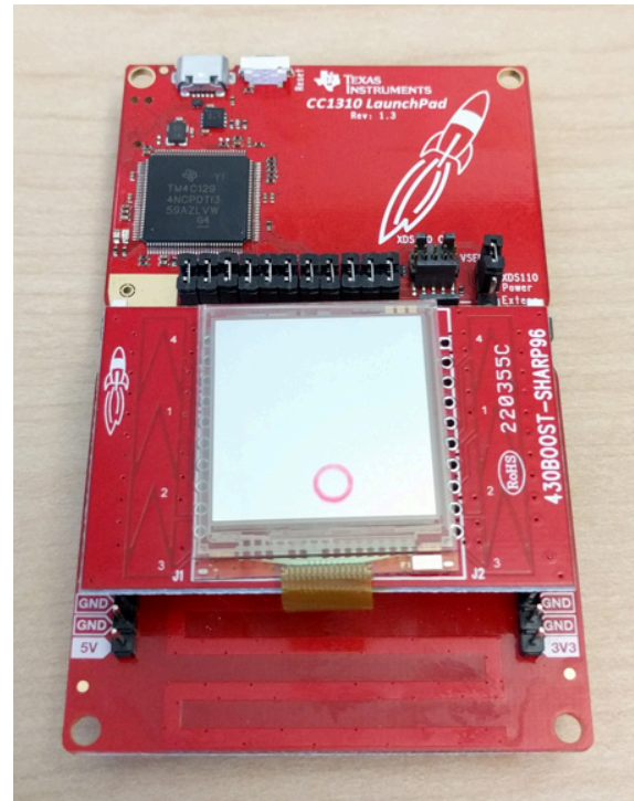
Figure 7. Fully Assembled System (Collector Node)
