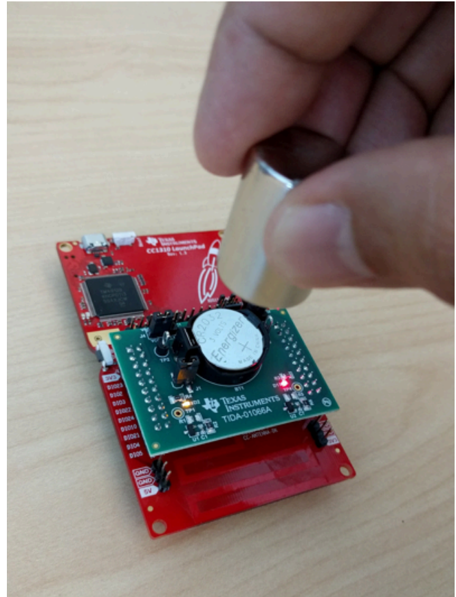
Figure 21. Magnet Top Test Setup (DCX0)
