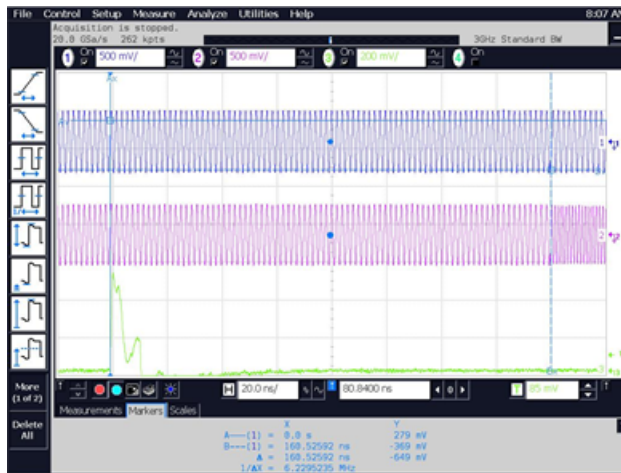
Figure 23. Transition From 500 MHz to 800 MHz
