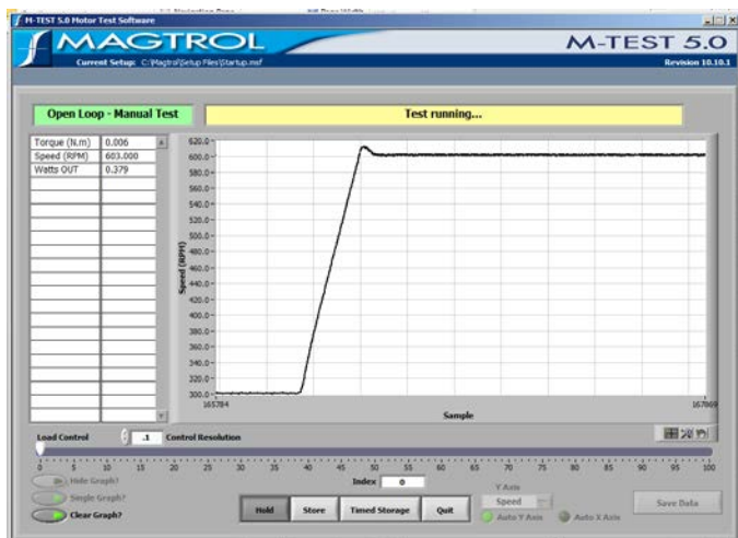
Figure 82 Speed ramp increase from 300 RPM to 600 RPM @ 200 RPM/sec, no brake
