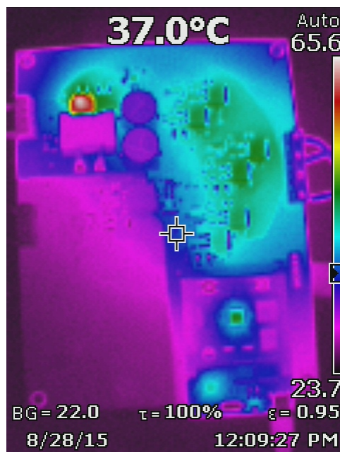
Figure 113 Thermal image - 1 Nm load, 1500 RPM, (233W/158W)
