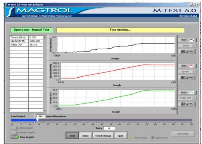
Figure 92 Speed response, RP34-313, 48V, 14% brake load
