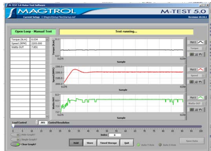
Figure 89 RP34-313 motor, 48V, detail of speed increase from 200 RPM to 2200 RPM @ 500 RPM, showing overshoot in speed response
