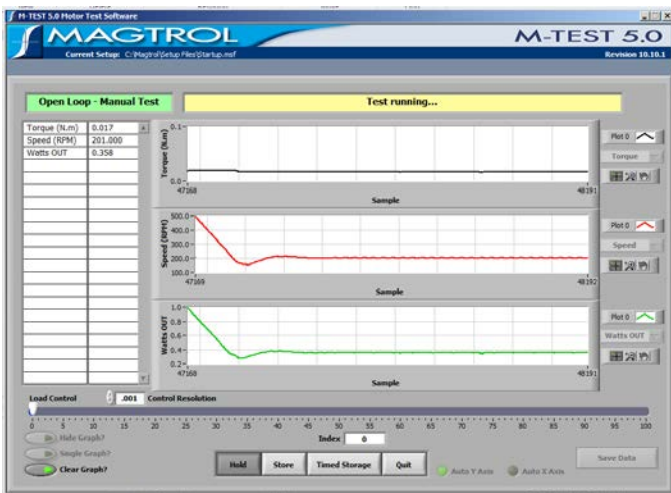
Figure 91 Detail of speed decrease showing overshoot in speed response
