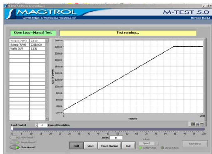
Figure 83 Speed ramp from 200 RPM to 2000 RPM @ 200 RPM/sec, no brake
