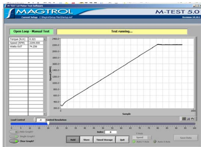
Figure 84 Speed ramp from 200 RPM to 2000 RPM @ 200 RPM/sec, 0.33 Nm load (77W)
