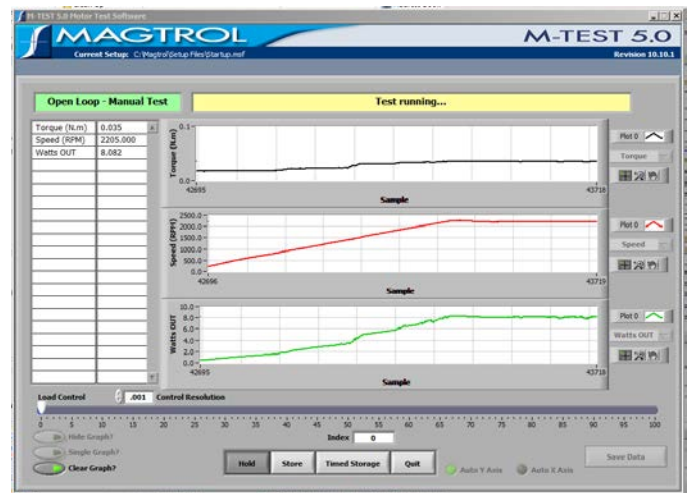
Figure 88 RP34-313, speed increase from 200 RPM to 2200 RPM @ 500 RPM/sec, no brake
