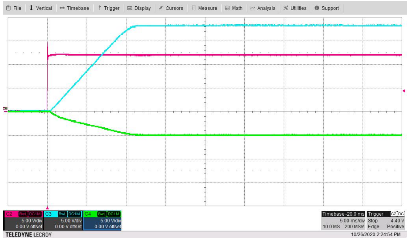
Figure 4-1. Start-up Sequence for +18V1 (Blue) and -5.1V1 (Green) With Vin = 12 V (Red)
