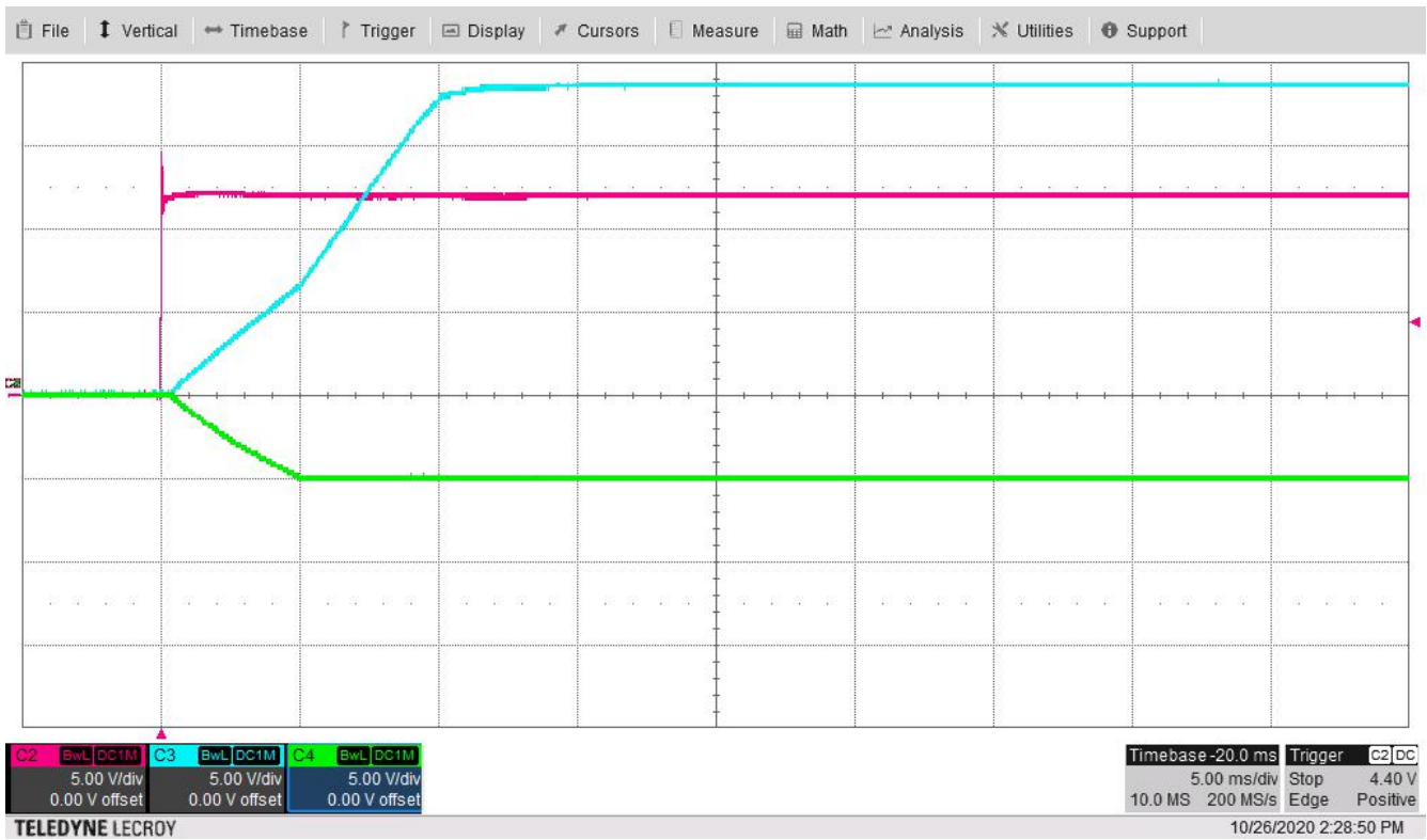
Figure 4-2. Start-up Sequence for +18V1 (Blue) and -5.1V1 (Green) With Vin = 12 V (Red)
