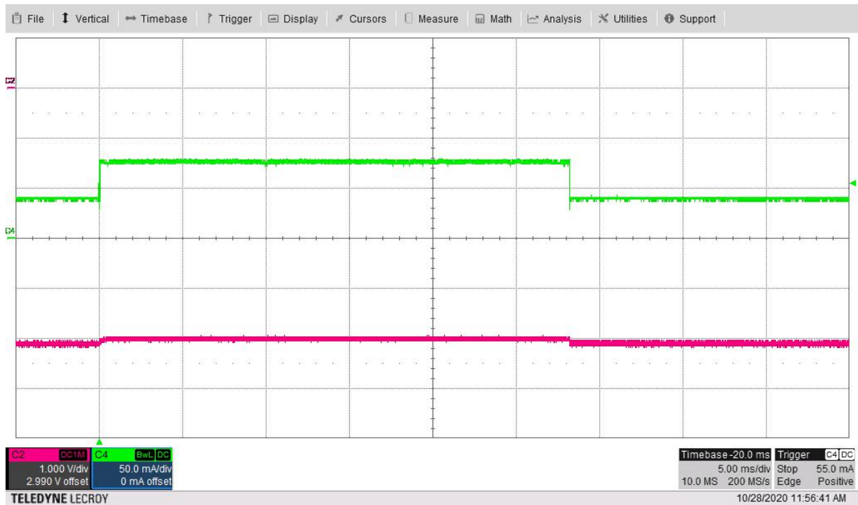
Figure 4-18. 50% Load Transient (38 mA to 75 mA, Green) on 18V1 (Red) for Vin = 12 V
