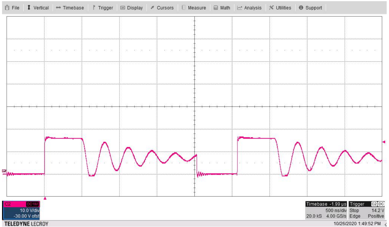
Figure 4-8. FET Switch Node Voltage at TP3 With V_{in} = 7\text{ V} and no Loads
