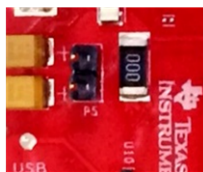
Figure 14. Current Measurement Point
