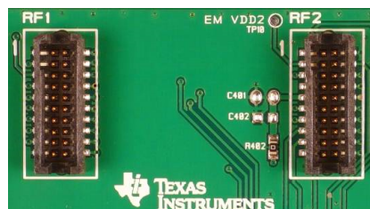
Figure 18. SmartRF06EB EVM Connectors RF1 and RF2
