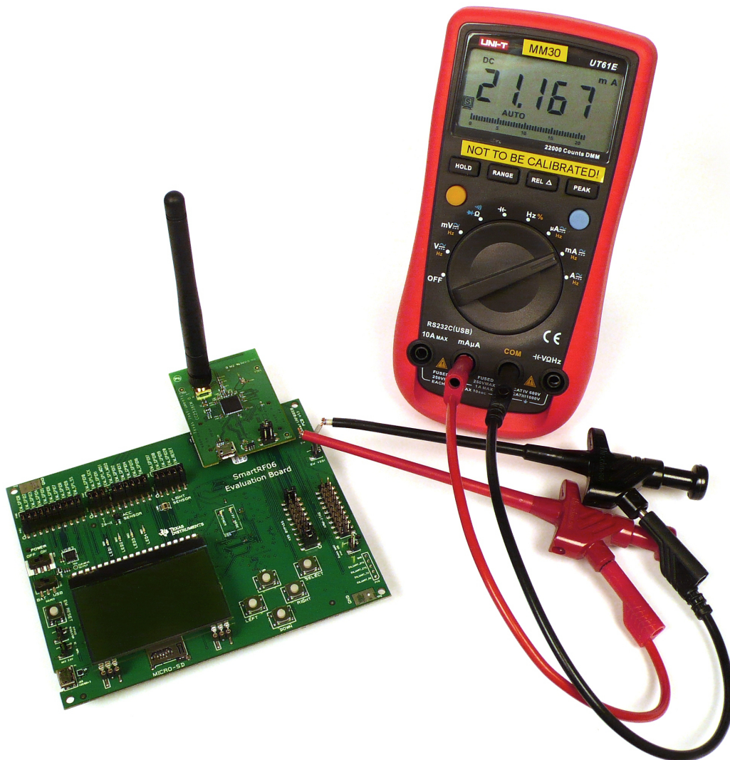
Figure 23. Measuring Current Consumption Using Jumper J503
