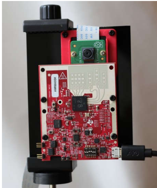
Figure 3. Camera and Radar Sensor Module Built With IMX219 and IWR6843ISK
