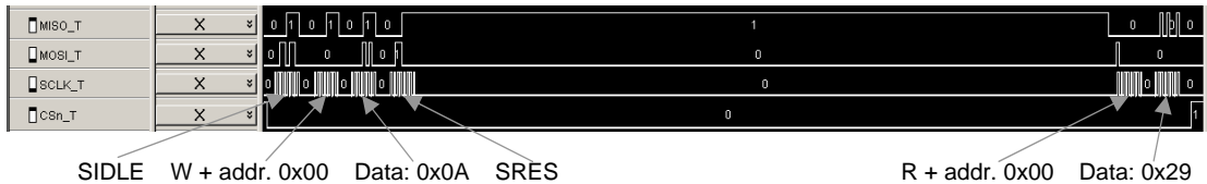
Figure 10. Several SPI Accesses with CSn Kept Low
