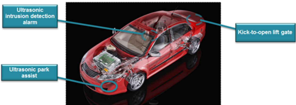
Figure 1. Ultrasonic Sensors in Passenger Vehicles
