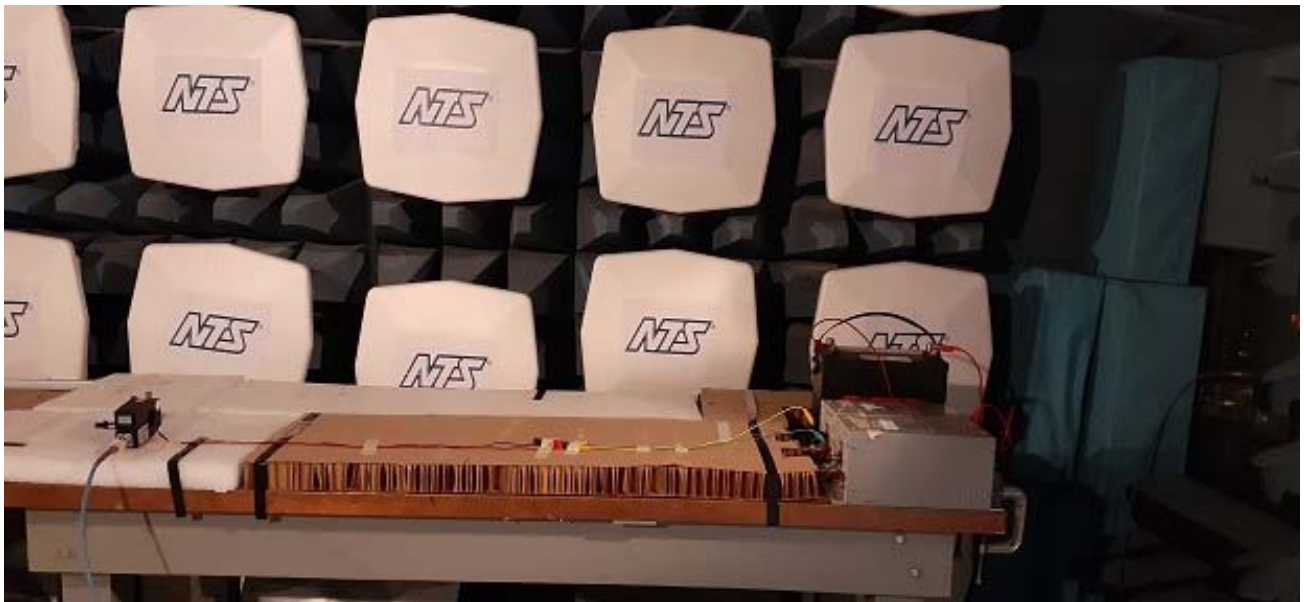
Photograph 7 CE 150 Khz-245MHz current@5cm test set up
