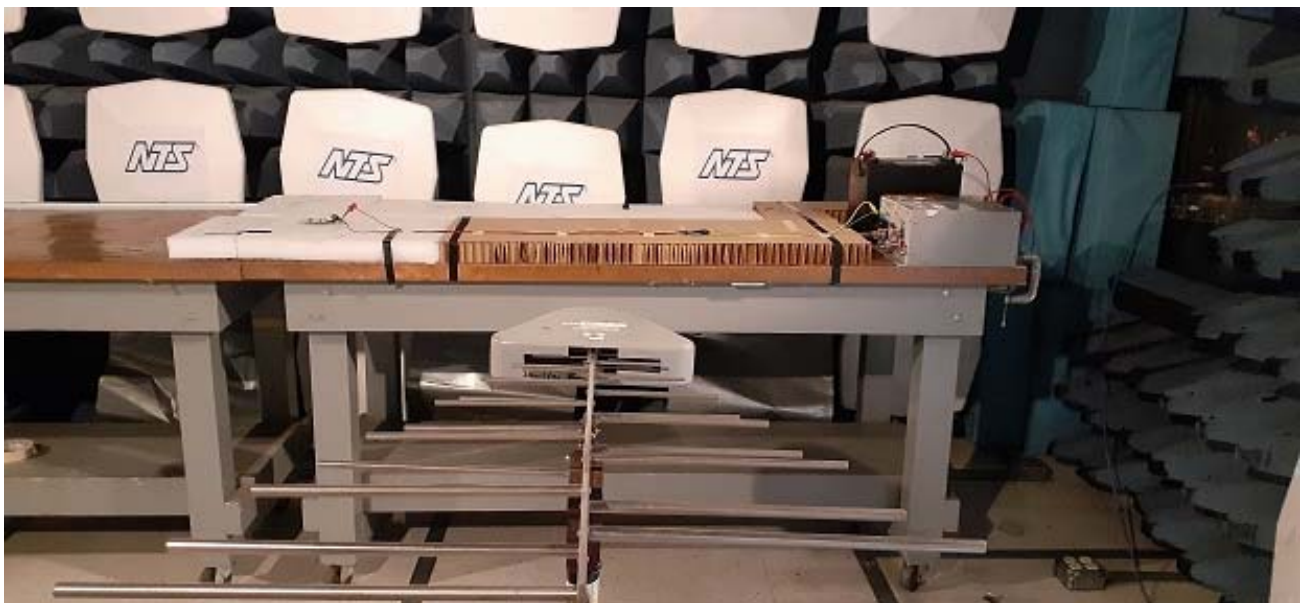
Photograph 4 CISPR 25 RE 200MHz-1GHz horizontal test set up
