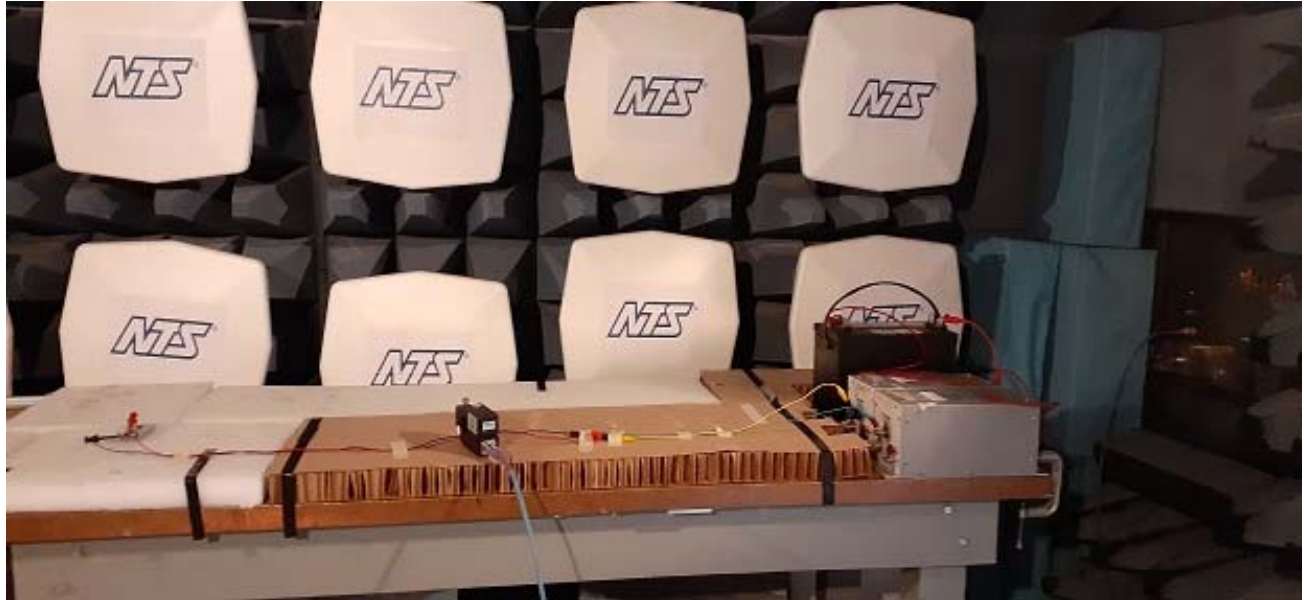
Photograph 8 CE 150 kHz-245MHz current@75cm test set up
