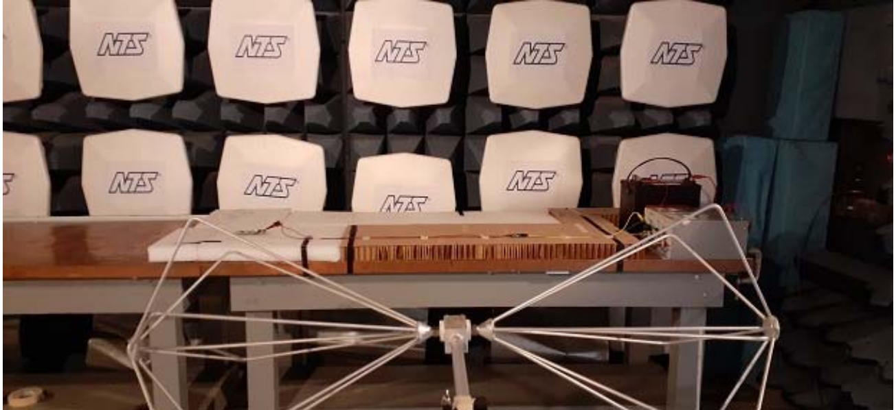
Photograph 2 CISPR 25 RE 30-200MHz Horizontal test set up
