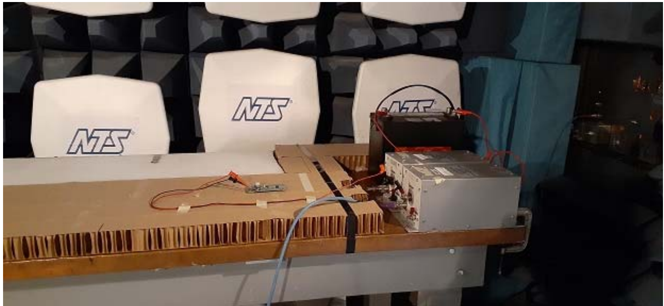
Photograph 9 CE 150Khz-108MHz Voltage HS test set up
