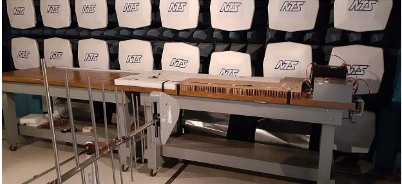
Photograph 5 CISPR 25 RE 200MHz-1GHz Vertical test set up
