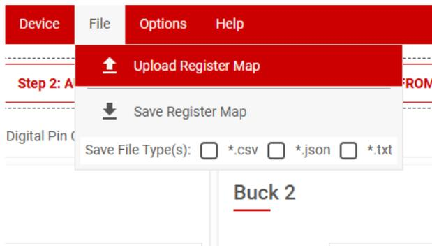
**Figure 4-10. Save and Load Register Options**
