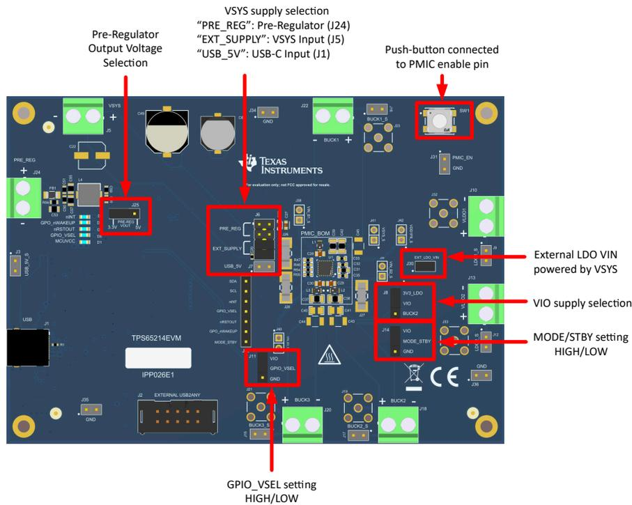
**Figure 3-4. TPS65214EVM Header Configurations**
