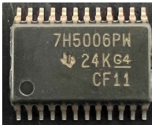
Figure 1-1. TPS7H5006-SEP Device Photo
