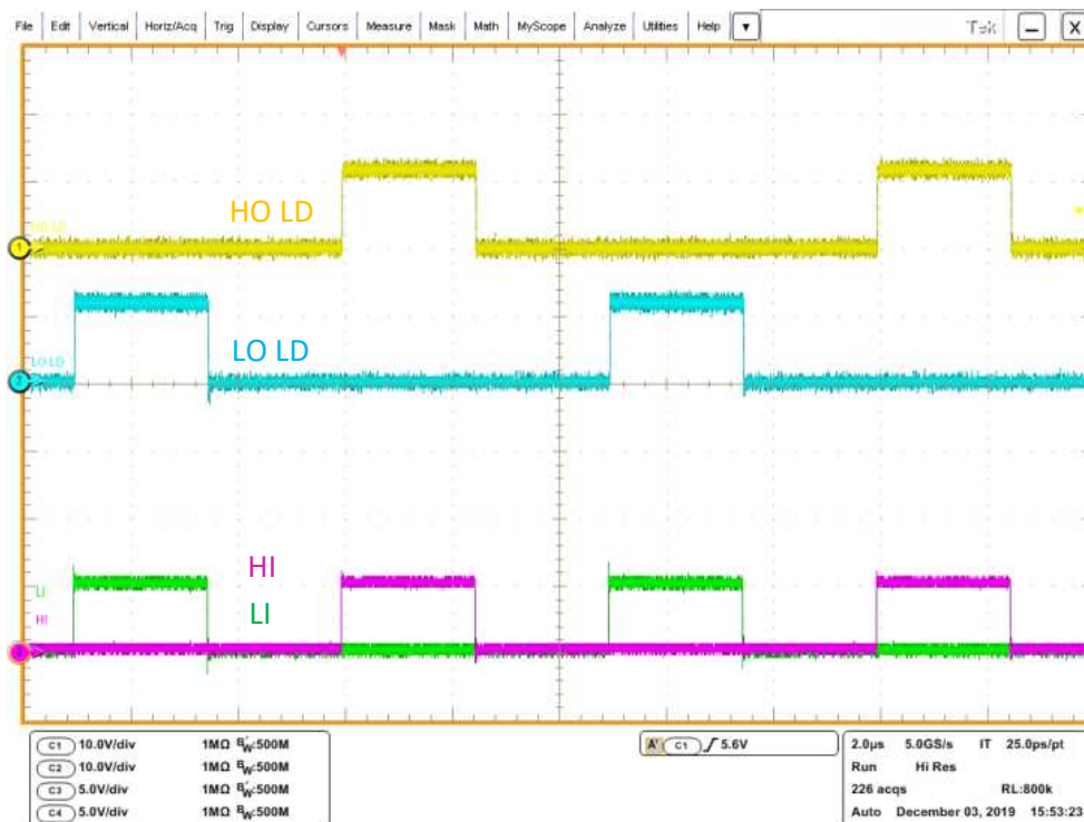
Figure 2. Example Input and Output Waveforms (Green and Magenta are PWM Inputs, Yellow and Blue are Driver Outputs)
