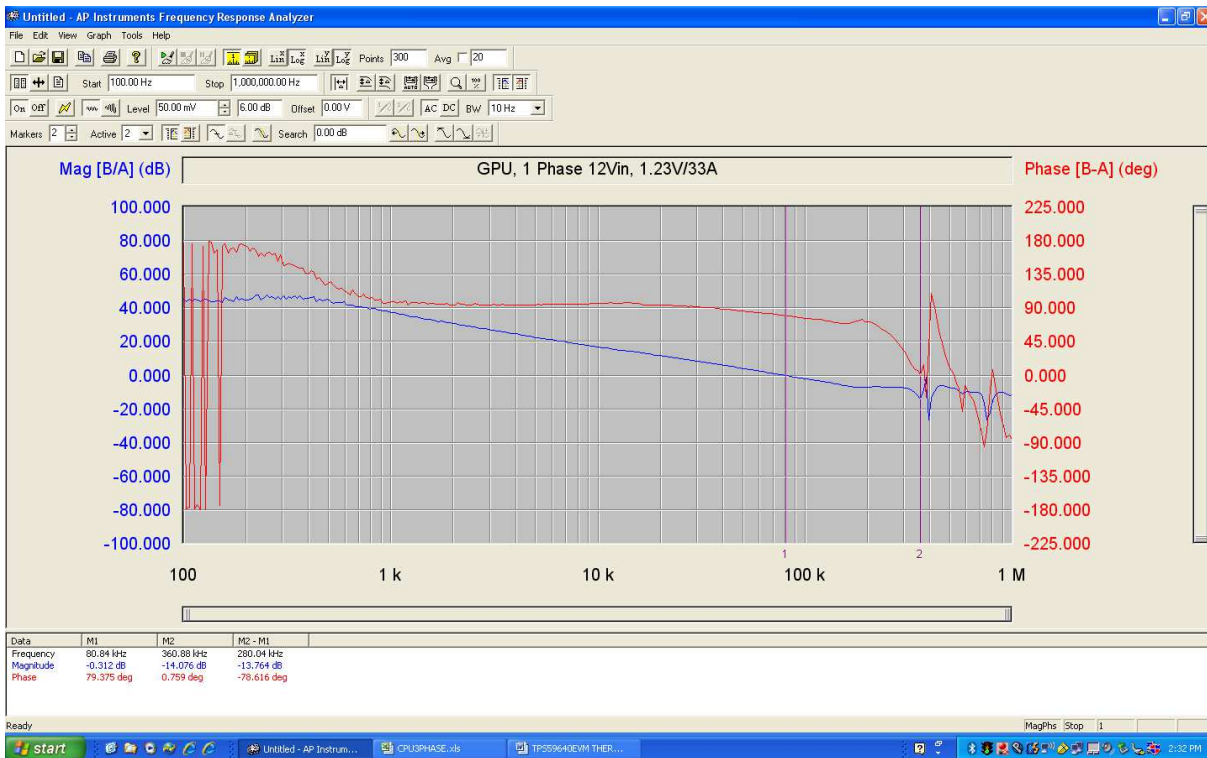
Figure 71. GPU1 Bode Plot at 12Vin, 1.23V/33A
