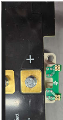
Figure 7-3. Interface Board to Connect Gate Driver EVM to BM3 Power Module
