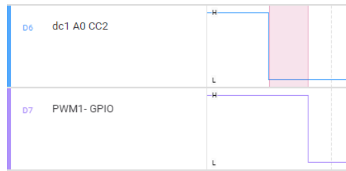
Figure 3-2. Delay between PWM and GPIO
