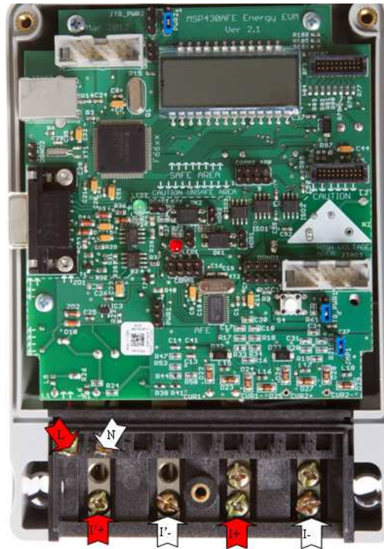
Figure 16. Top View of the EVM With Test Setup Connections
