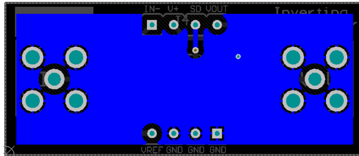
Figure 32. Inverting Comparator Bottom Layer
