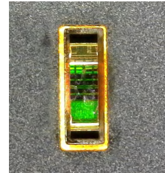
Figure 2-5. Image of FPCB With OPT4001YMN-Q1 Mounted, Receiving Light Through the Cutout with a Rectangular Shape
