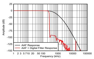
Figure 2-7. Combined Anti-Alias Filter and Digital Filter Response
