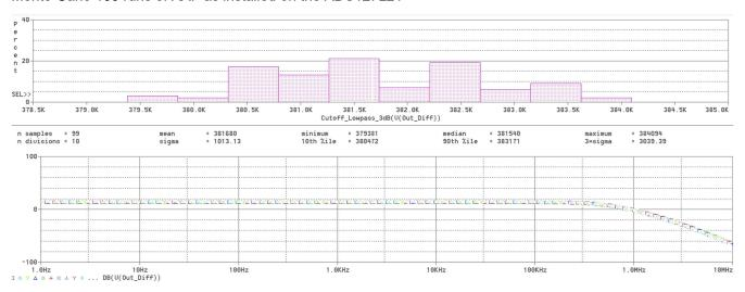
Figure 2-3. Monte-Carlo Simulation with the New AAF
