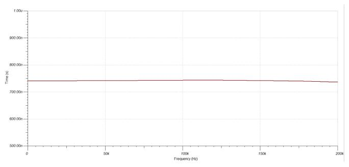
Figure 2-5. Simulation of the AAF Group Delay after Modification
