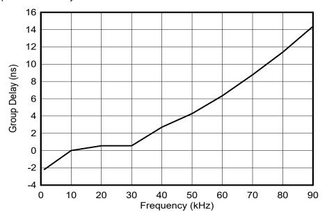
Figure 2-11. Group Delay of the Signal Chain (Normalized to 10kHz)
