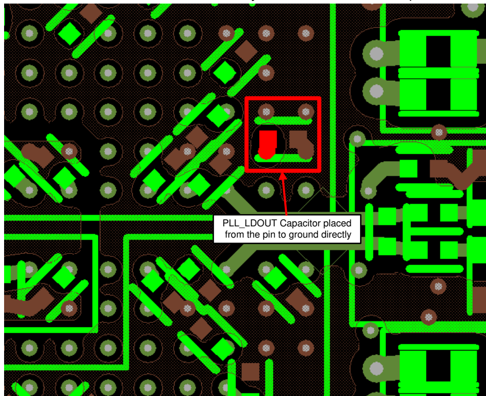
Figure 6-8. PLL_LDOUT 0.1- \mu F Capacitor Routing From Pin J19 (PLL_LDOUT) to Pin J18 (VSSPLLCLKREF)
