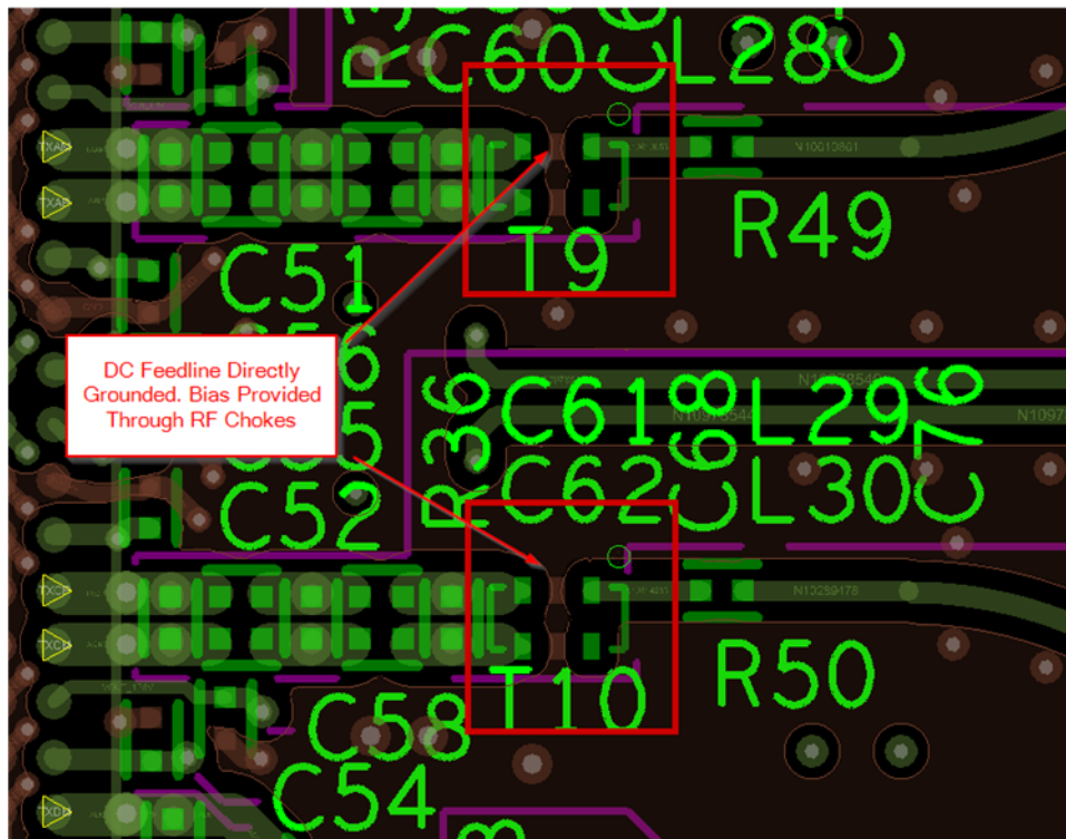
Figure 8-4. Current Implementation: DC Feed Line Directly Grounded. Bias Provided Through RF Chokes
