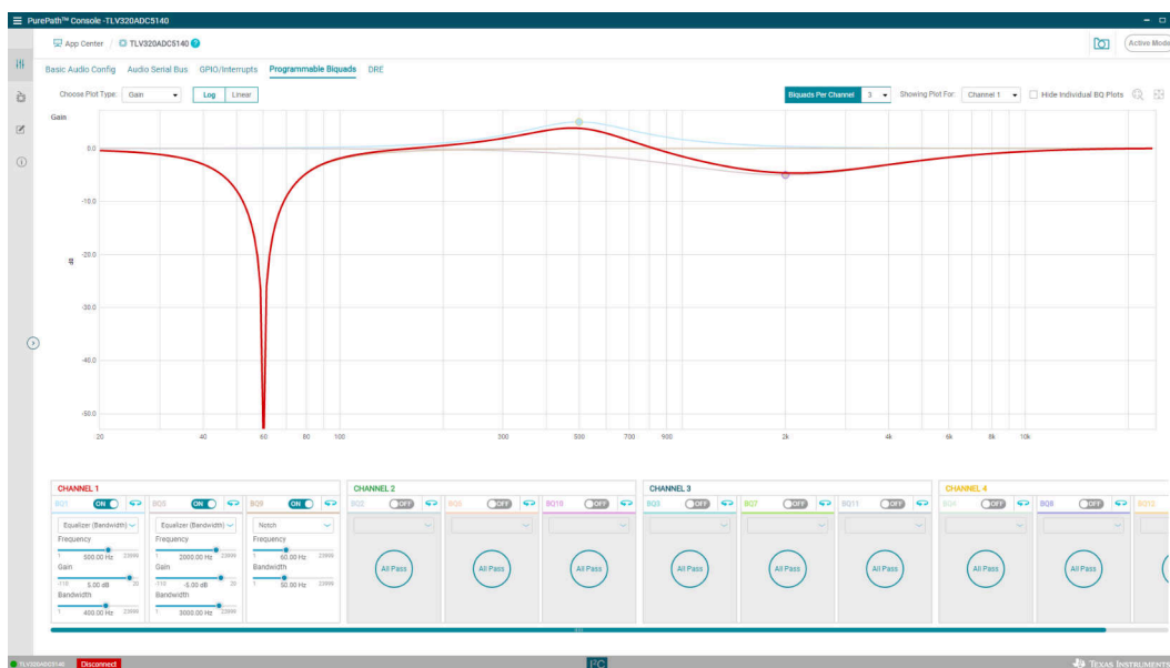
Figure 3-2. PurePath™ Console Programmable Biquad Filter Example
