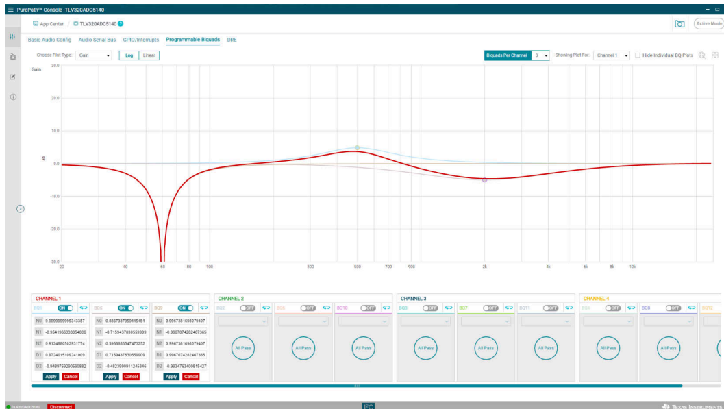
Figure 3-3. PurePath™ Console Programmable Biquad Filter Example Showing the Computed Coefficients in Normalized Floating Point Format
