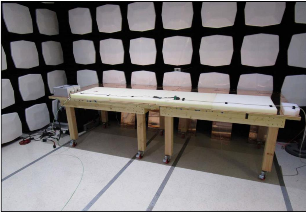
図 8. Conducted Emissions Test Setup
