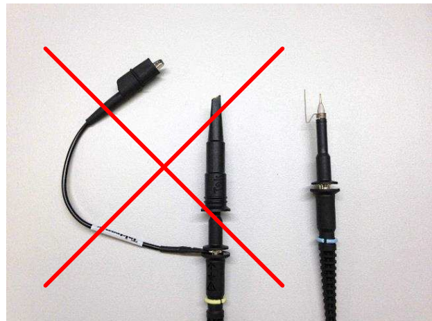
図 19. Probe With Long Ground Lead and Alligator Clip vs Probe With Ground Spring
