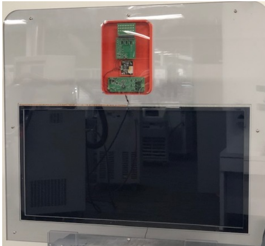
Figure 16. TIDA-020011 Controlling a Larger Demonstration Featuring LED Matrix Control and SPD-Smartglass™
