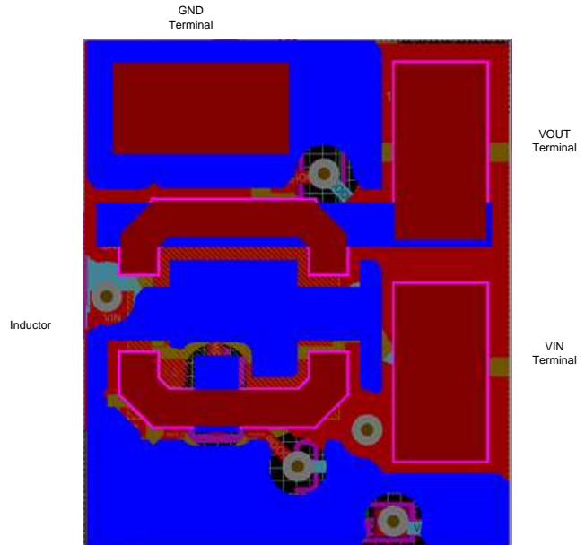
13. PMP15040 PCB Layout: Bottom Layer
