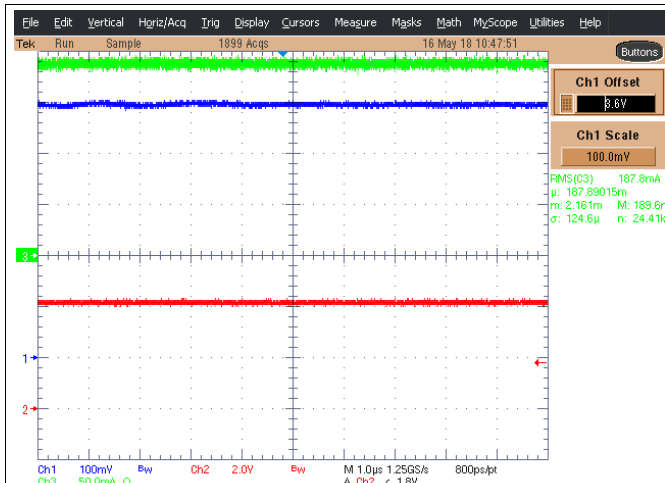
図 43. VBAT1=4.2V, VBAT2=3.3V, Boost Switching Waveform
