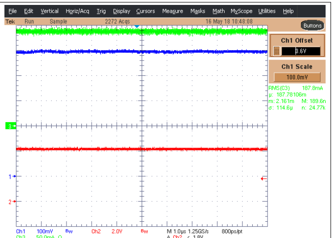
図 44. VBAT1=4.2V, VBAT2=3.6V, Boost Switching Waveform
