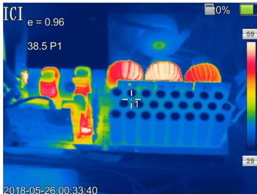
図 76. Thermal Image of the TIDA-01604 at 240-V AC Input With 6.6-kW Load
