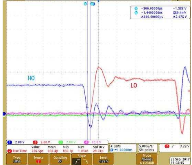
12. Dead Time Measurement Done at V_{IN} = 0 Showing High-to-Low Transition Dead Time of 640 ps
