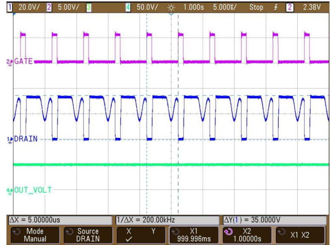
61. Gate, Drain, and Output Voltage Waveforms for Synchronization to 200-kHz External Clock
