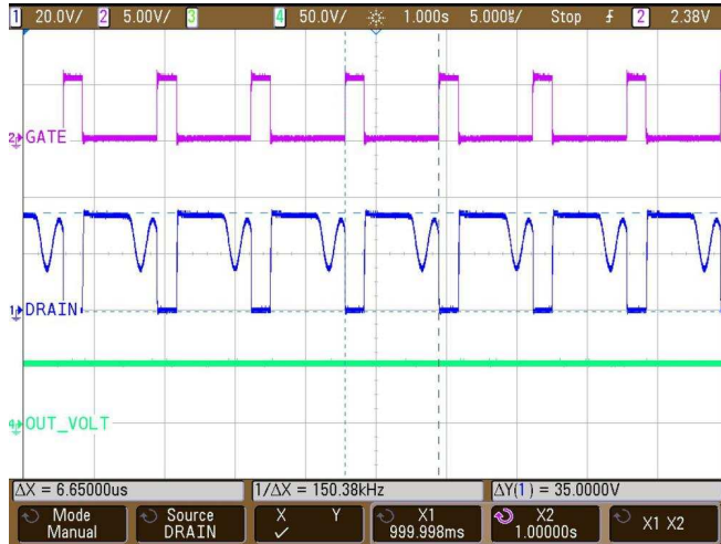
60. Gate, Drain, and Output Voltage Waveforms for Synchronization to 150-kHz External Clock
