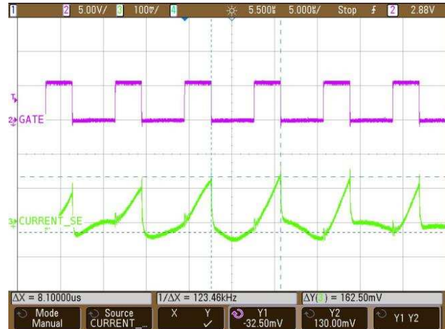
29. Current Sense Waveform With Gate Drive at Full Load ( V_{OUT}= 80\text{ V} , I_{OUT}= 160\text{ mA} )
