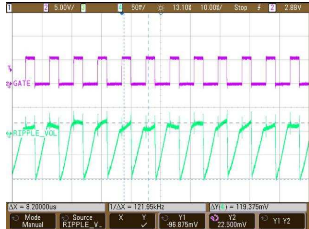
Figure 31. Output Voltage Ripple at the Negative Rail at 80-V Full Load
