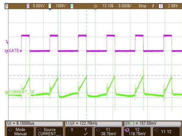
Figure 36. Current Sense Waveform With Gate Drive at Full Load ( V_{OUT} = 50\text{ V} , I_{OUT} = 250\text{ mA} )
