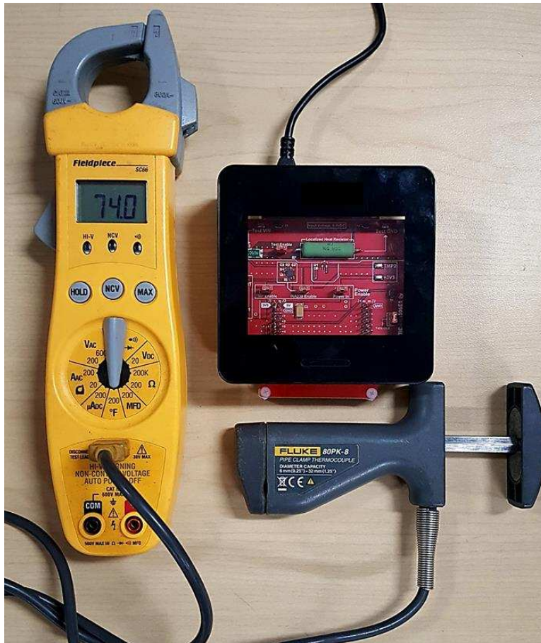
Figure 42. Load Offset From Ambient Test Setup In Thermostat Case
