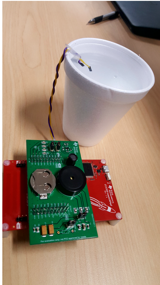
図 23. Test Setup of Water Leak Detection
