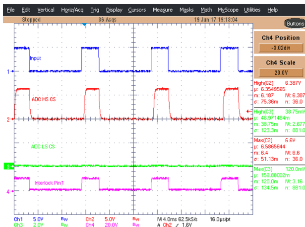
図 45. TIDA-01445 Short Circuit to Ground at Pin 2
