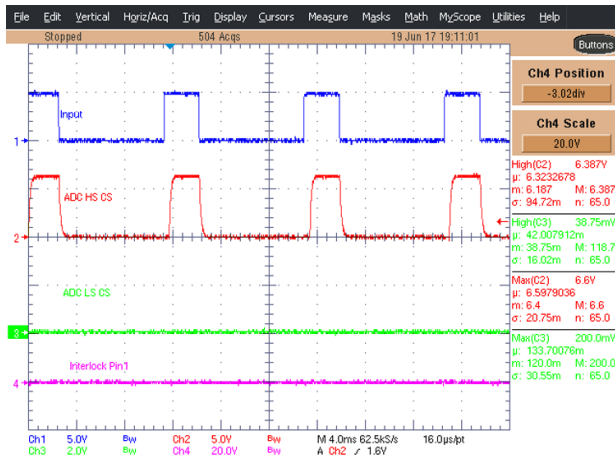
図 44. TIDA-01445 Short Circuit to Ground at Pin 1
