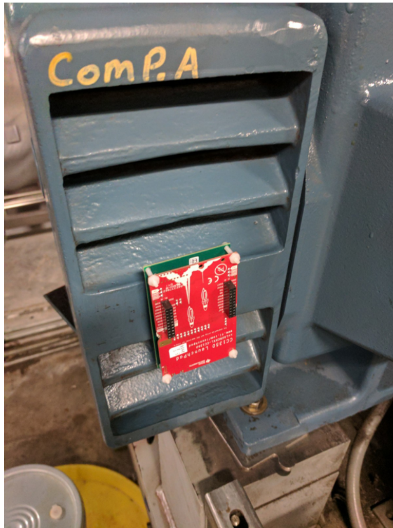
図 14. Reference Design Coupled to Motor
