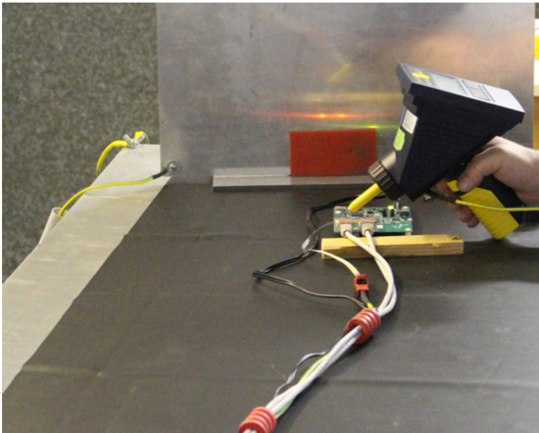
Figure 62. IEC61000-4-2 Test Setup for TIDA-00204 (Picture of 6-kV CD)
