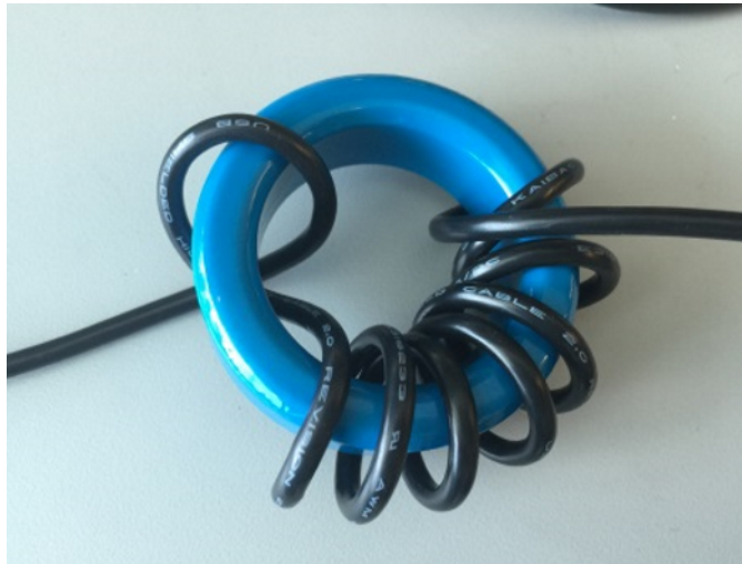
Figure 17. USB Cable Around Ferrite Bead
